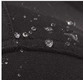
Durable Water Repellent (DWR) Finish
