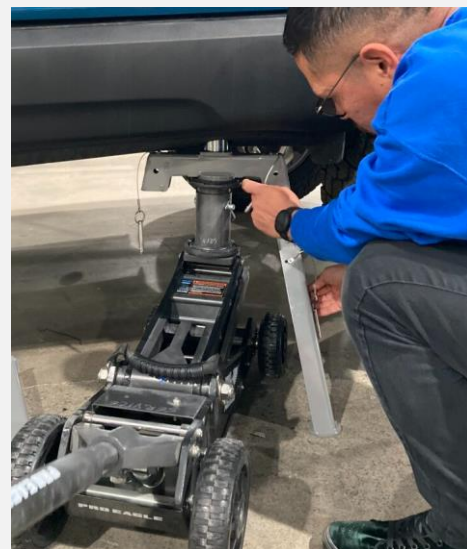
Installation des Wagenheberstandbeins
