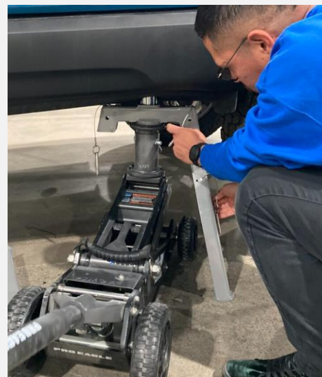
Jack Stand Leg Installation
