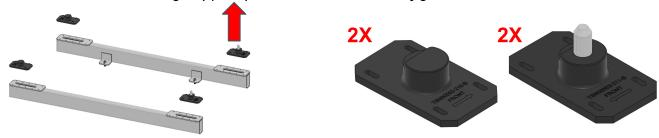
2. **INSTALL** 4x new rubber support pads provided in upgrade kit. Tighten bolts until snug.
