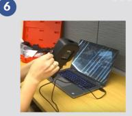
Connect your device to the PC using the USB cable included in the kit. This will allow a two-way connection between your device and PC.
